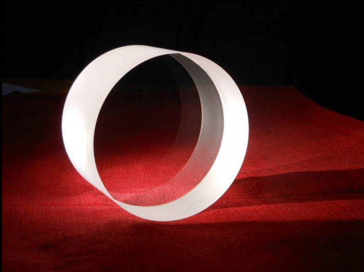
Sapphire mirrors (High Q in cryogenic temperature)
