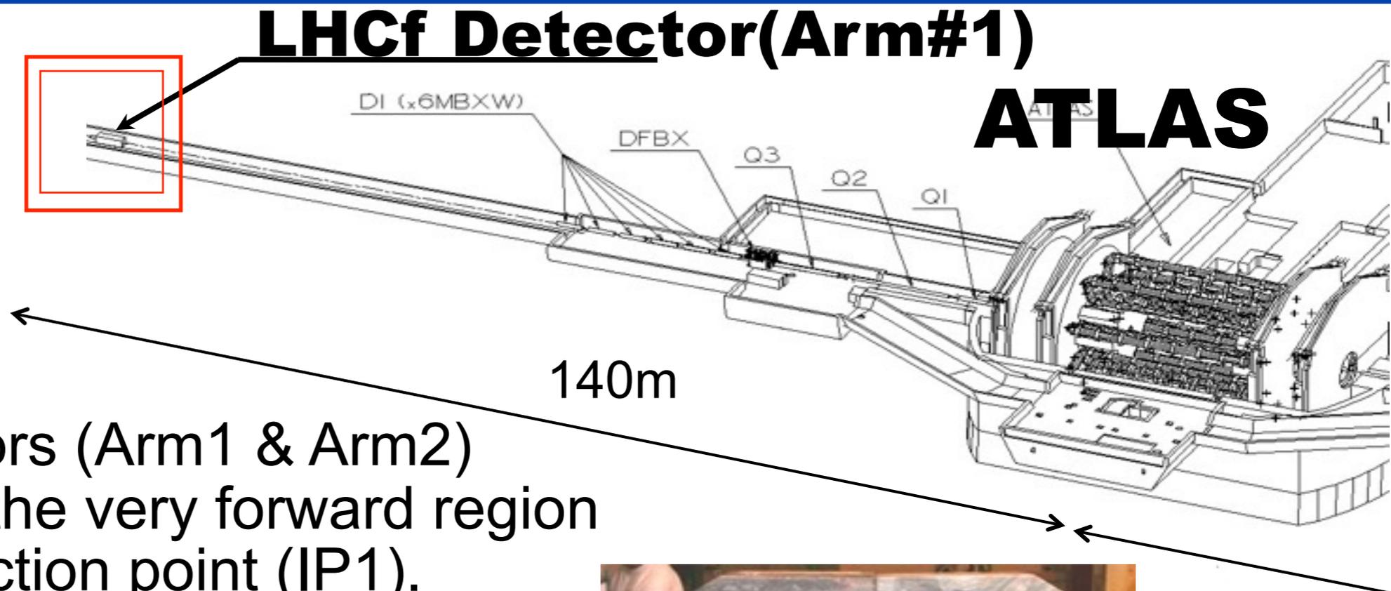
Two LHCf detectors (Arm1 & Arm2) are installed into the very forward region of the LHC interaction point (IP1). LHCf can measure neutral particles ( $\gamma$ ,  $n$ ) at the rapidity range  $\eta > 8.4$ .
