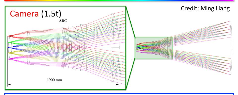
The telescope (lens+mirror coating+detector) is optimized to have high UV (320-390nm) throughput;
