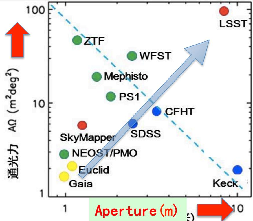
**WFST ( $A\Omega = 29.3$ ) is a powerful survey machine, with a cost only 1/50 of LSST.**
