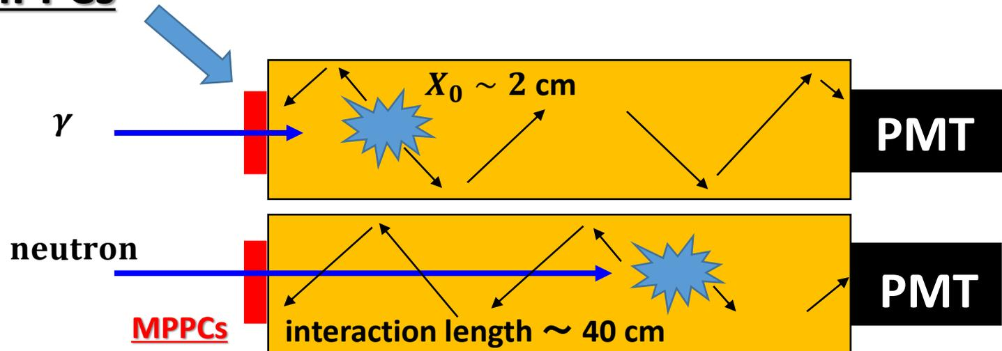
Measure the depth with the time difference  $\Delta T \equiv T_{MPPC} - T_{PMT}$
